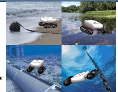
Top to bottom: LASR’s screw-based propulsion system and AI-based path planning for survey missions
